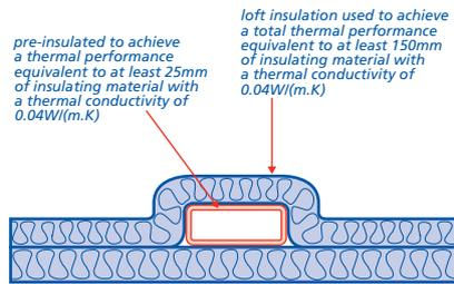
Condensate drains located outside the insulated part of the home should be insulated to prevent freezing.
